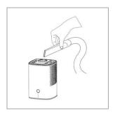
Clean out any remaining dust or hair inside the purifier using a vacuum hose of dry cloth. DO NOT use water or liquids to clean the purifier.
