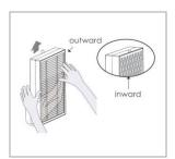
Remove any packing from the new filter elements and take notice of the inward and outward sides of the filter element.
