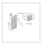
Before using the air purifier for the first time, open the base and remove both filters. Make sure you altogether remove any packaging from each filter element, or the product will not function correctly. (See page 9).
