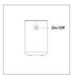
The indicator light will be blue and flash for about one second when the power adaptor is first connected to the purifier, indicating the purifier is in standby mode. Press the on/off button once to turn on the device; the indicator light will now be blue; the device will operate in the default mode (sleep) fan speed.
